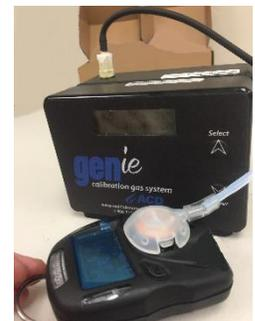
ACD Ozone Calibrator used with UNI O<sub>3</sub>
