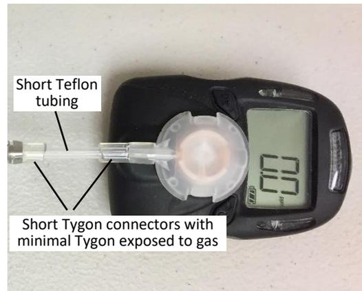
Exploded view showing tubing connections
