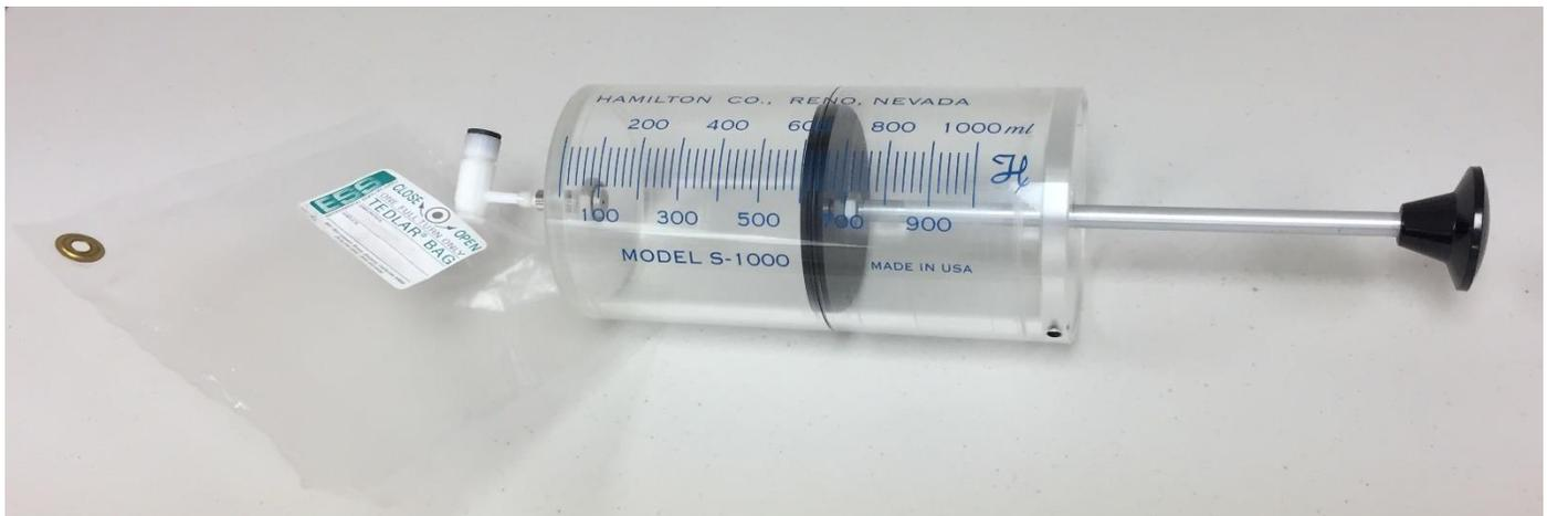
Gas dilution system using a Tedlar gas bag and a high-volume syringe
