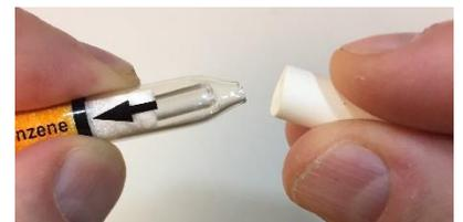
Grip tube close to end and snap off tip
