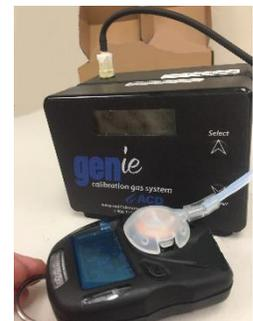
ACD Ozone Calibrator used with UNI O<sub>3</sub>
